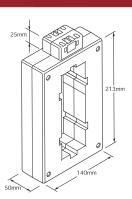
• Hole for M6 diameter screws or busbar mounting
